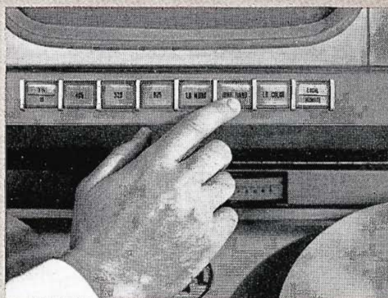
TR-70 has "instant selection" of high band or low band, color or monochrome.
