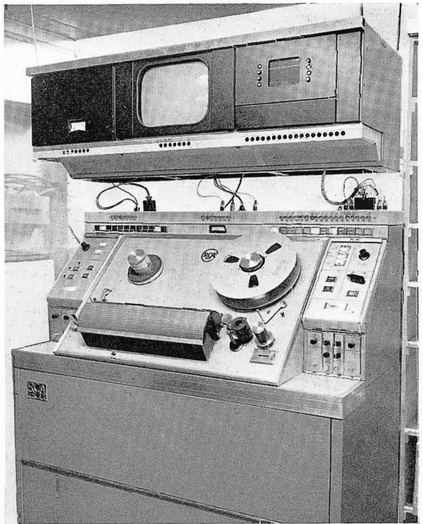
FIG. 18. TR-22 tape recorder modified to permit frequent transporting of equipment in TV mobile unit. A monitoring section duplicating that shown here (at top) is permanently mounted in mobile van.
