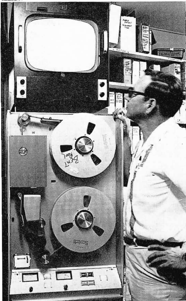
FIG. 17. TR-3 tape player is indispensable in color taping operations.
