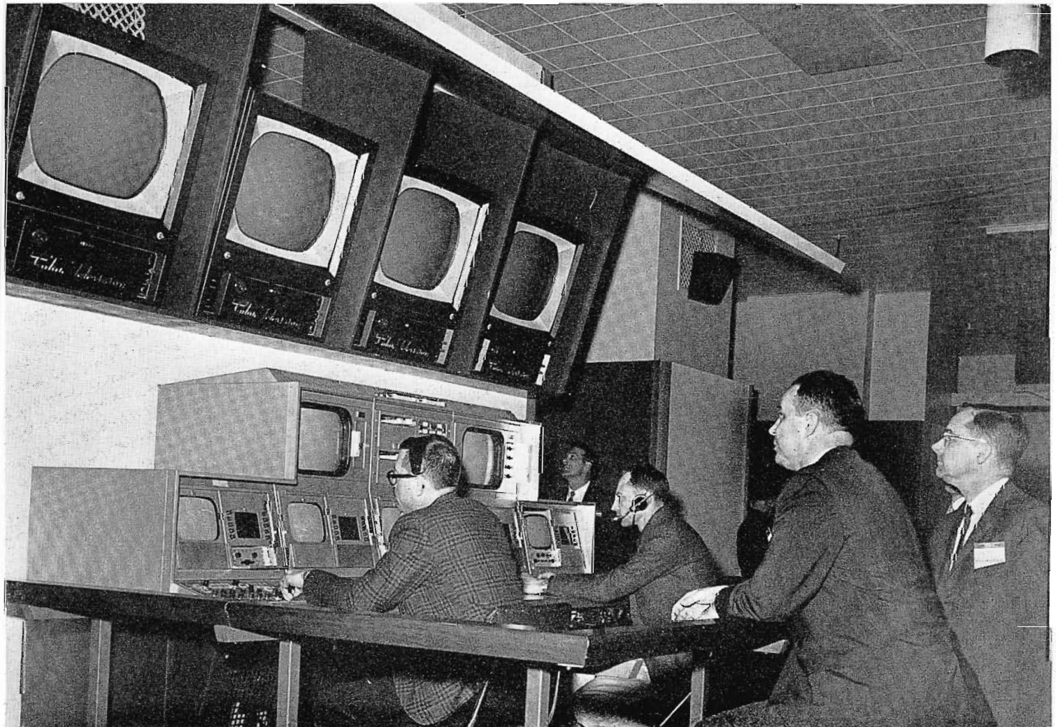
Color Central provided video switching, effects and distribution, serving as intermediary between the TK-42s and 22 monitoring locations.
